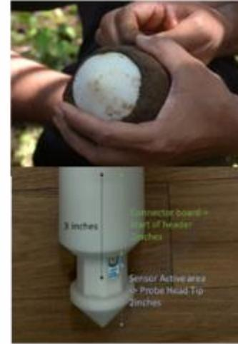
Soil-Proto Probe test setup
