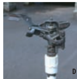
Figure 10.15 —(A) Both overhead and basal sprinkler systems feature rotating “spinners” or (B) stationary nozzles which, in addition to full circles, are (C) available in quarter, half, and three-quarters coverage. (D) Because of their greater coverage, rotating-impact (Rain Bird®-type) sprinklers (E) are commonly used in outdoor growing areas. Photos by Thomas D. Landis, illustration by Jim Marin.
