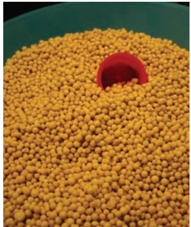
Figure 11.7 —Polymer-coated fertilizers occur as round “prills” in which nutrients are encapsulated by a plastic coating that controls the rate of nutrient release. Photo by Douglass F. Jacobs.
