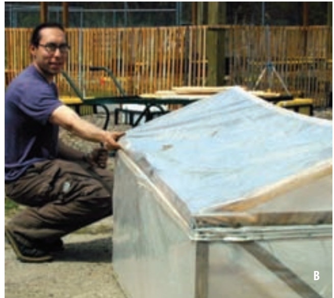
Figure 4.11 —(A) Rooting cutting requires a specialized propagation environment because cuttings lack a root system. (B) The “poly propagator” is the most simple and inexpensive rooting chamber; this one being used by Shannon Wetzel is at the Salish Kootenai College Nursery in Montana. Illustration by Steve Morrison, photo by Tara Luna.
