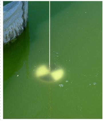
A secchi disk is a simple device used to measure the density of phytoplankton population (bloom). The depth at which the disk is no longer visible is the secchi disk value. Values of 6-9 cm indicates a moderate bloom. Values of 4 cm or less indicate a heavy bloom and extreme daily oxygen fluctuations would be expected. Increased aeration is necessary.
