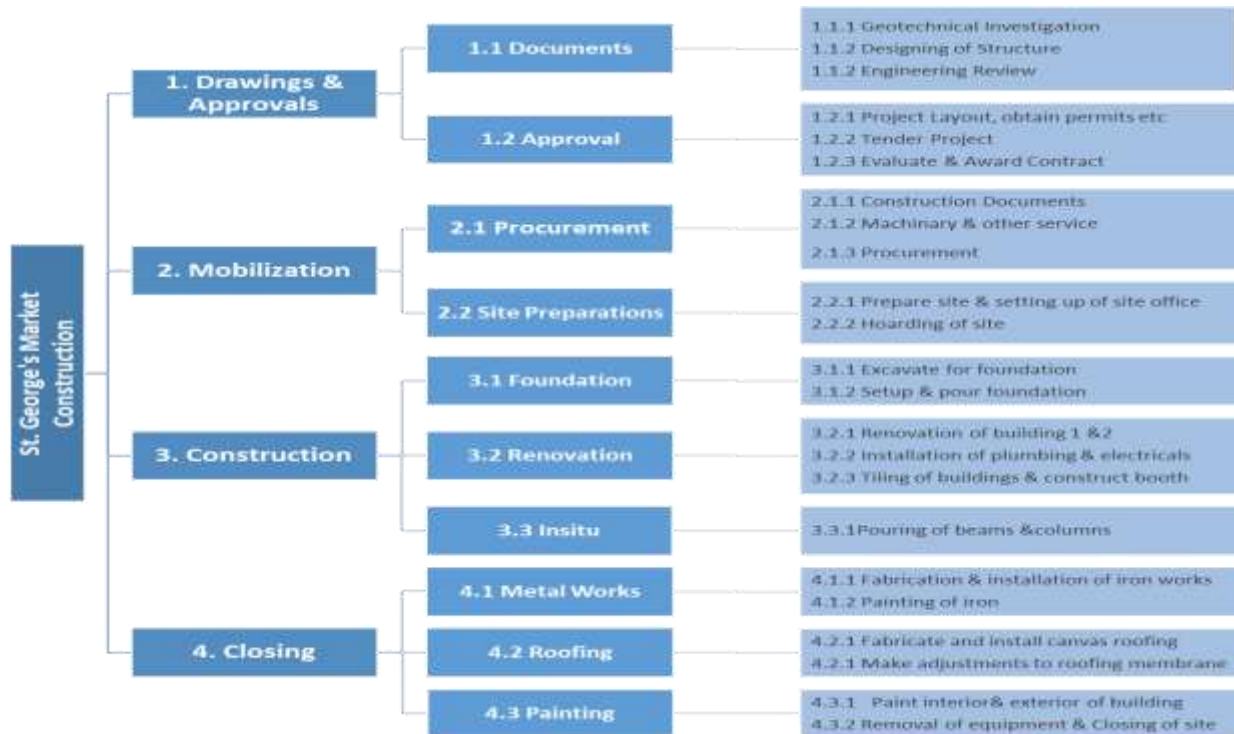
Figure 6 shows the WBS of the market project (Source: Compiled by author J. Victor)
