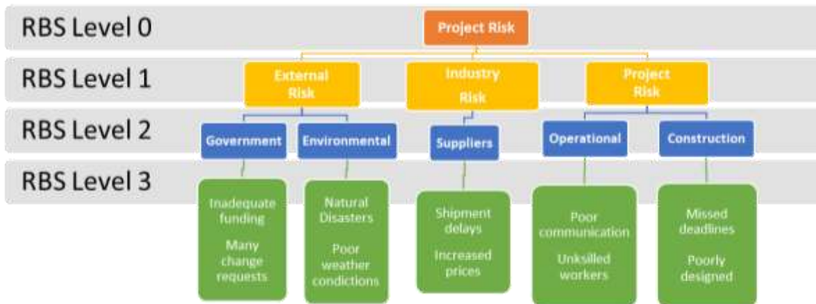
Figure 13 illustrates the RBS Risk Breakdown Structure for the St. George's Market Construction Project (Source: Compiled by J. Victor)
