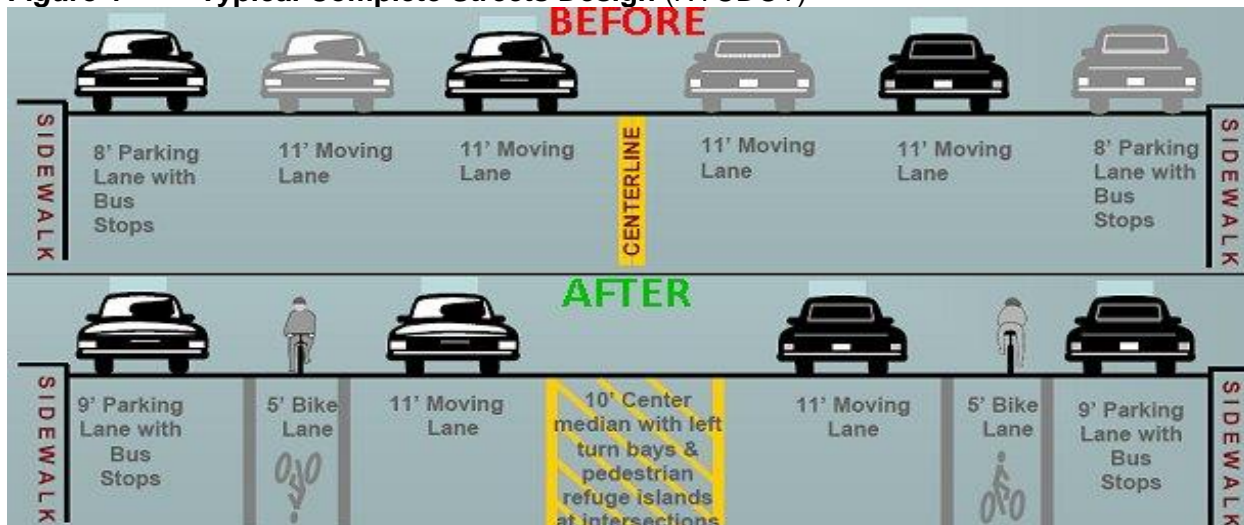
Figure 4 Typical Complete Streets Design (NYCDOT)
