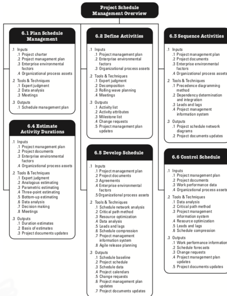
Figure 9 PMBOK Guide Project Schedule Management overview. Reprinted from A Guide to the Project Management Body of Knowledge (p. 174), Project Management Institute, 2017, Project Management Institute. Copyright 2017 by Project Management Institute, Inc.
